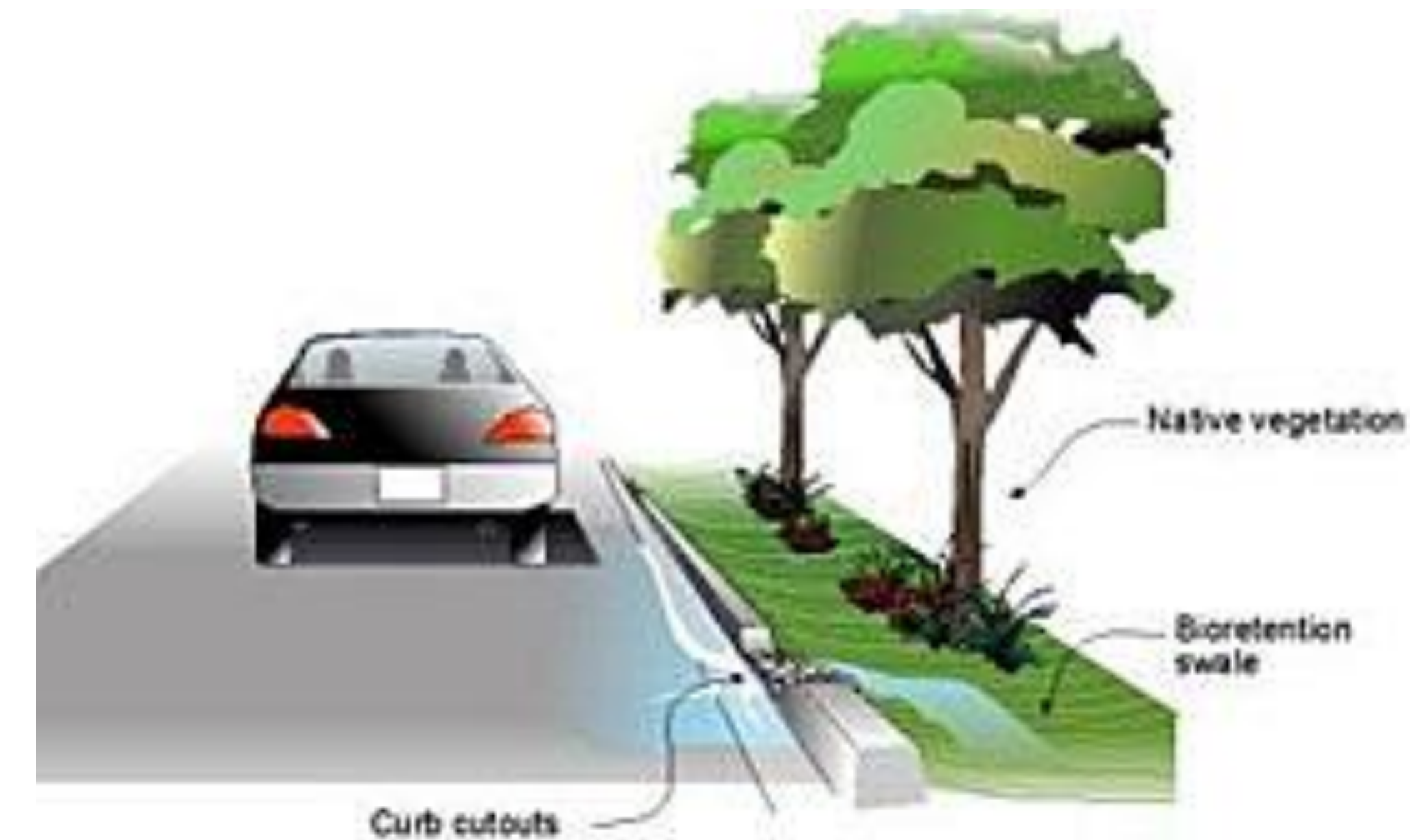
Example of curb cutout draining to roadside ditch to be installed. Photo Credit: Pierce County, Washington and AHBL, Inc.
