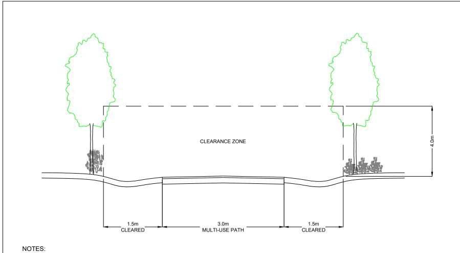
1. SURFACE MATERIAL TO BE DETERMINED ON A SITE SPECIFIC BASIS BY THE TOWN OF CALEDON.
