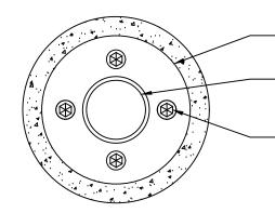
229mm DIA. x 13mm ALUM. BASE PLATE WITH 4-19mm DIA. HOLES
