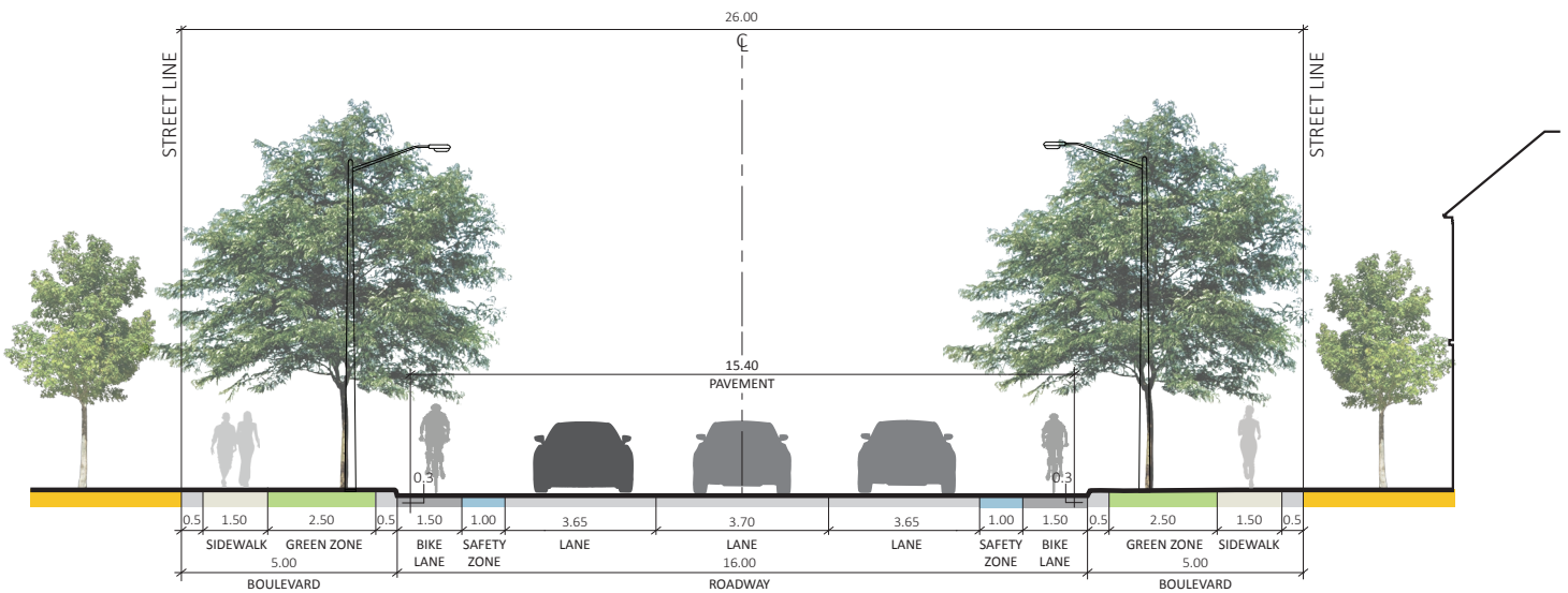
FIGURE 9 - Airport Road (26m R.O.W.) Cross-Section
