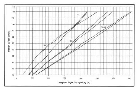
Figure 9.9.5: Intersection Sight Distance – Case B2, Right Turn from Stop, and Case B3, Crossing Maneuver (Calculated and Design Values Plotted)
