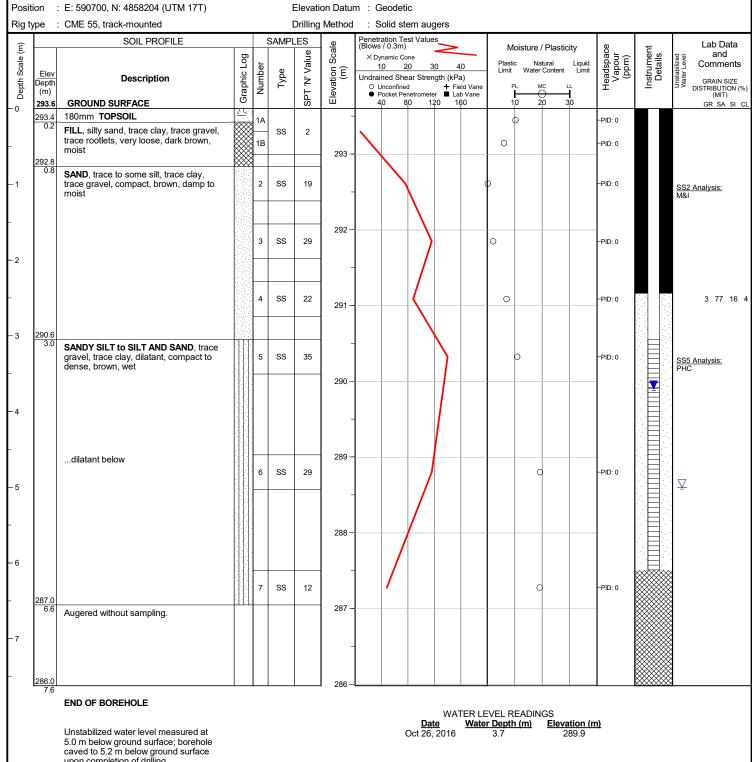
5.0 m below ground surface; borehole caved to 5.2 m below ground surface upon completion of drilling.
