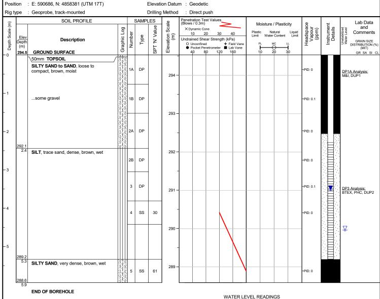
Unstabilized water level measured at 4.6 m below ground surface; borehole caved to 5.3 m below ground surface upon completion of drilling.
