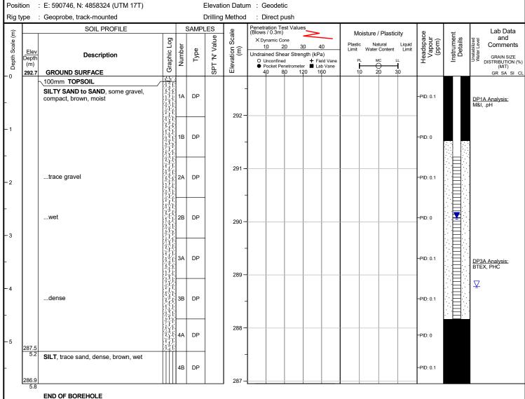
Unstabilized water level measured at 4.0 m below ground surface; borehole caved to 4.6 m below ground surface upon completion of drilling.
