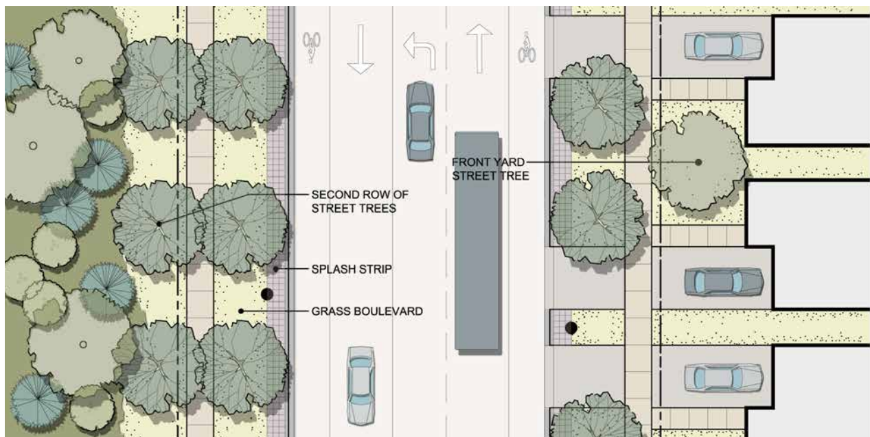
Figure 6.4.1a – Section A2-A2: Conceptual Spine Road treatment west of Collector Road D (27.0m ROW) with 2 thru lanes, left turn lane, on-street bike lanes, and street trees in grass boulevard adjacent to NHS lands and front driveway single-detached dwellings (looking west).
