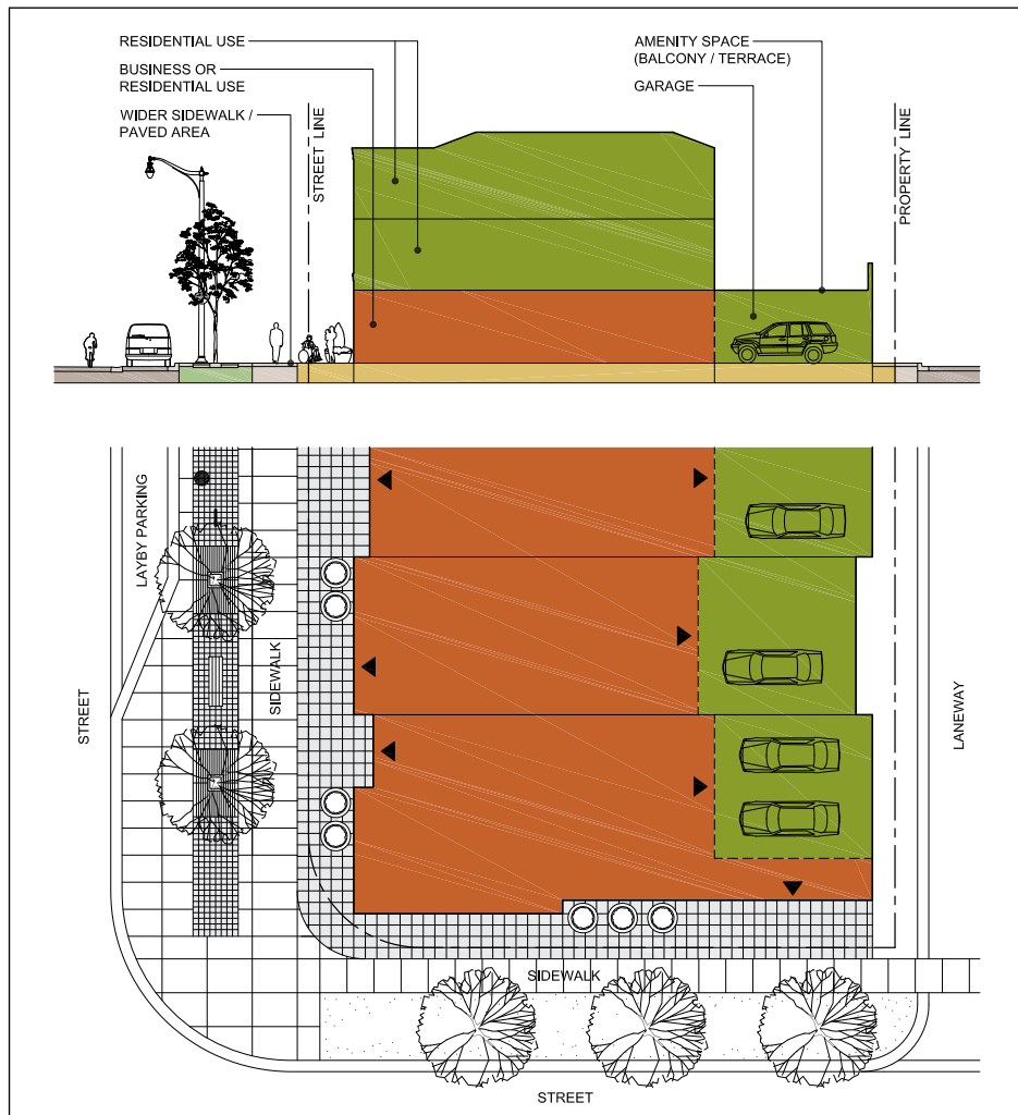
Figure 8.5.2s – Conceptual cross-section and plan siting for typical live-work townhouses.
