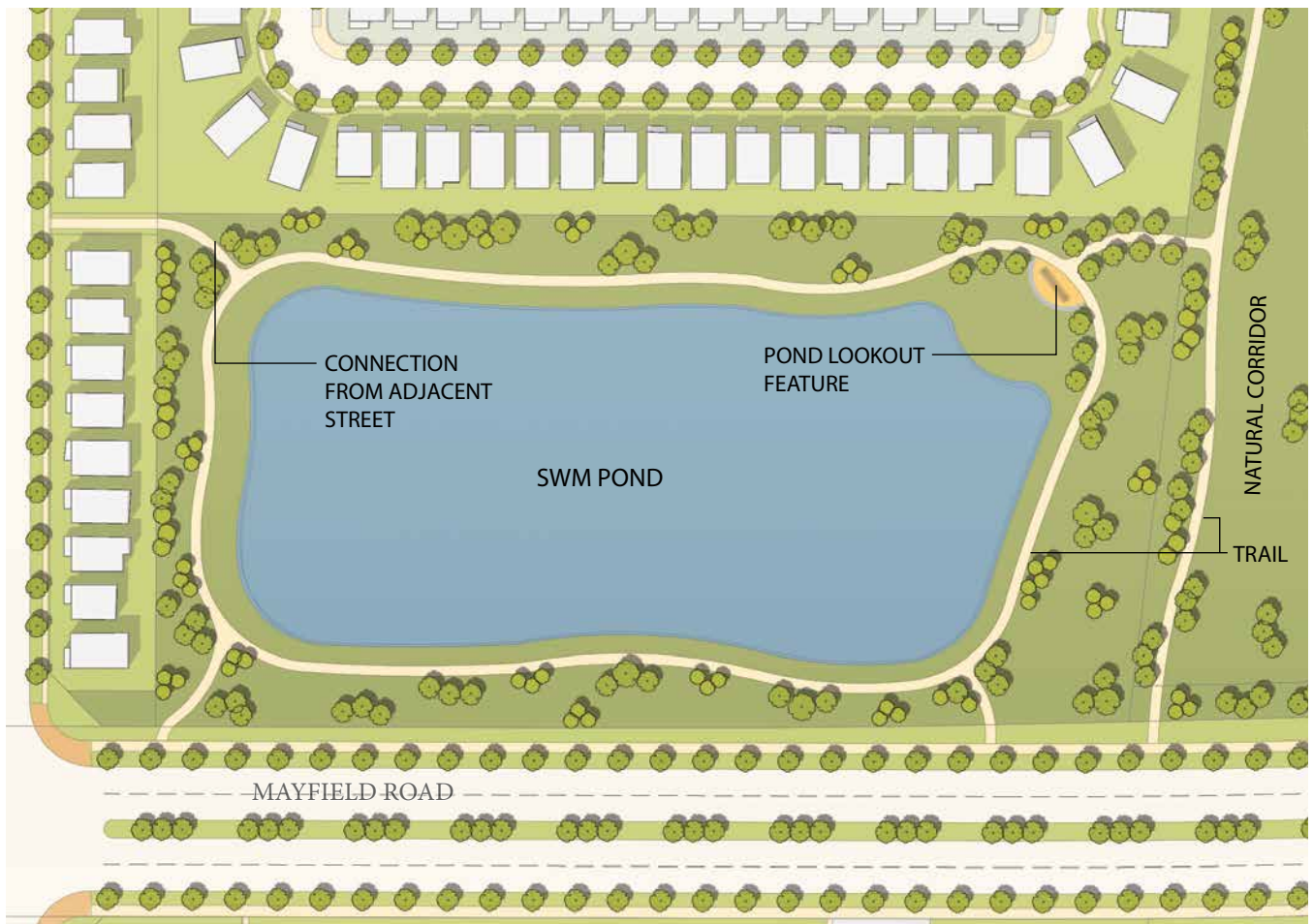
Figure 5.3e – Conceptual plans showing the layout of potential SWM ponds along Mayfield Road. The top image shows a typical design response, and below shows a more urban treatment associated with adjacent proposed commercial block.
