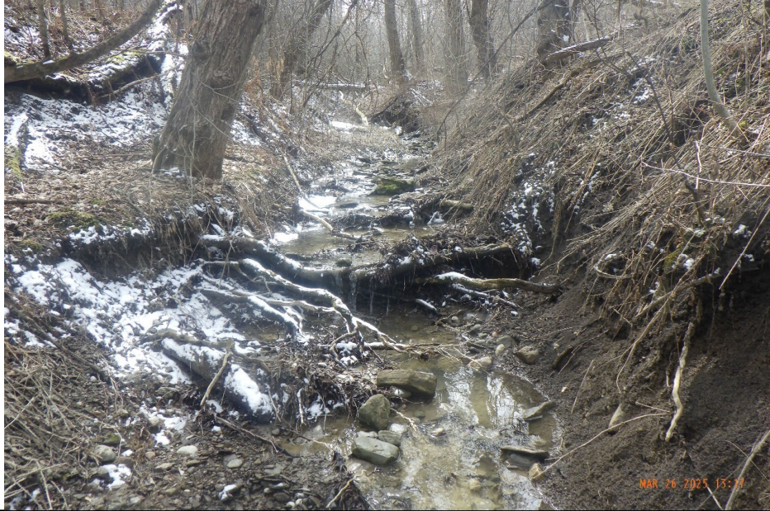
Photograph taken facing upstream of the first rooted knickpoint observed. The height was 0.30 m.
