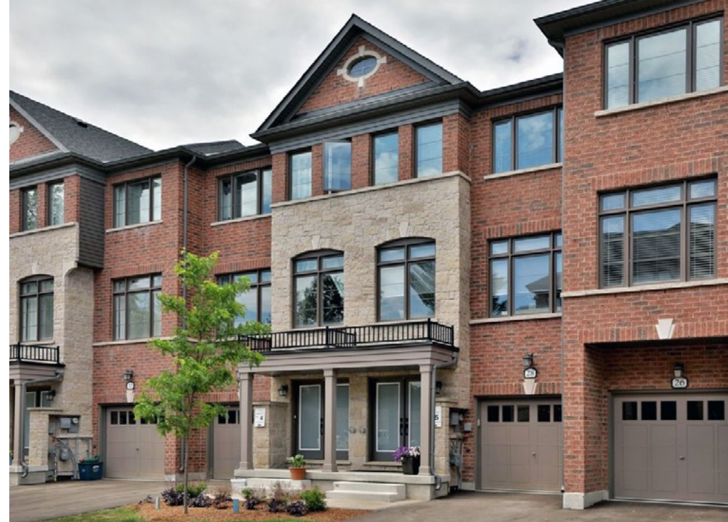
The overall townhouse block composition should display massing and design continuity while achieving adequate streetscape variety
