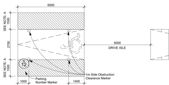
NOTE: A- PROVIDE AN ADDITIONAL 1500mm FOR PARKING SPACE WIDTH WHEN OBSTRUCTIONS OCCUR BETWEEN THE FRONT AND REAR 1000mm
