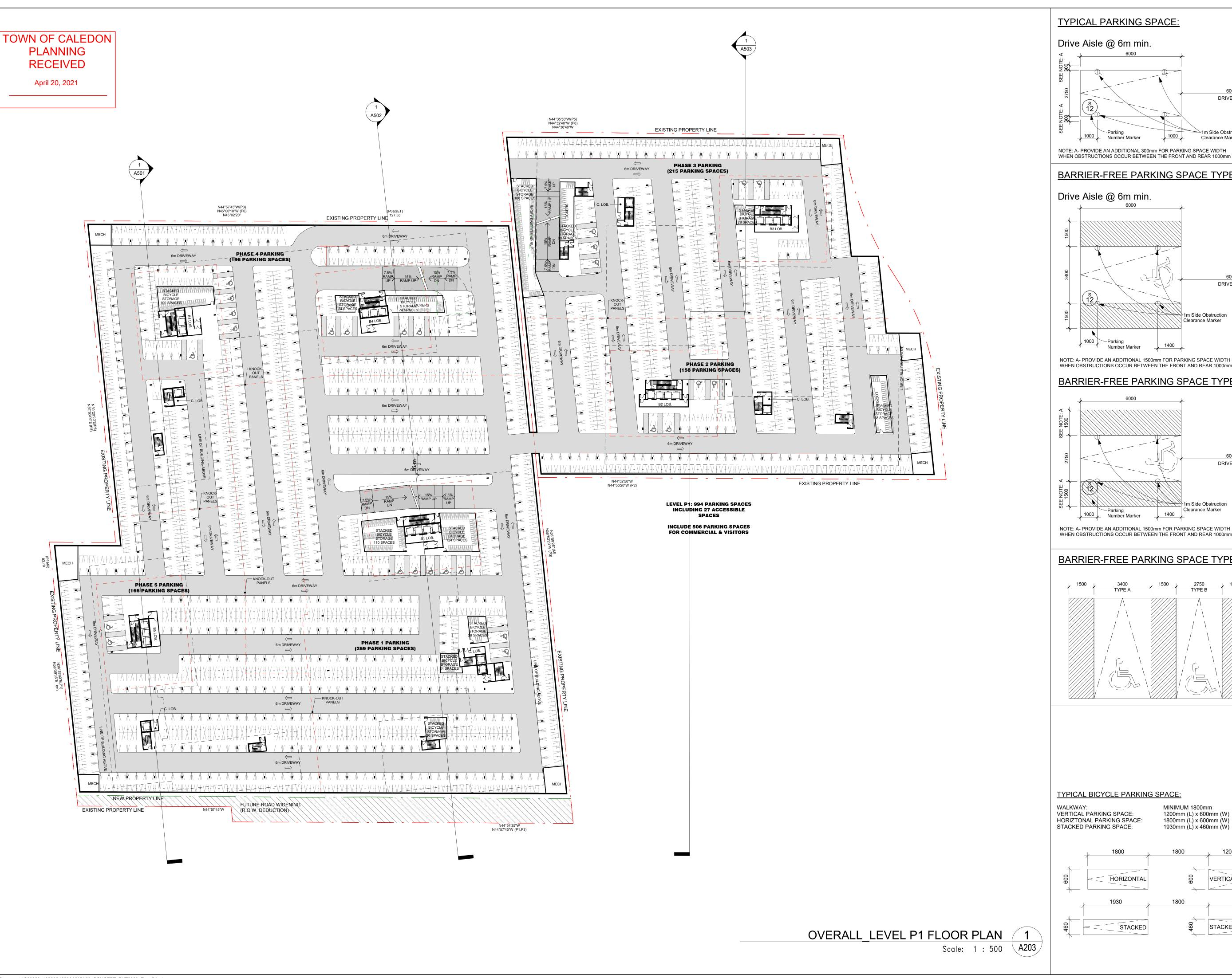
**TYPICAL PARKING SPACE:** Drive Aisle @ 6m min. DRIVE ISLE <sup>→</sup>1m Side Obstruction NOTE: A- PROVIDE AN ADDITIONAL 300mm FOR PARKING SPACE WIDTH WHEN OBSTRUCTIONS OCCUR BETWEEN THE FRONT AND REAR 1000mm BARRIER-FREE PARKING SPACE TYPE A:
