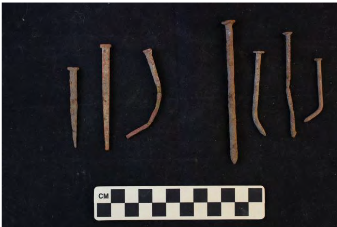
Image 135: Location 29; a representative example of nails. L to R: machine cut nails (x3), wire drawn nails (x4).
