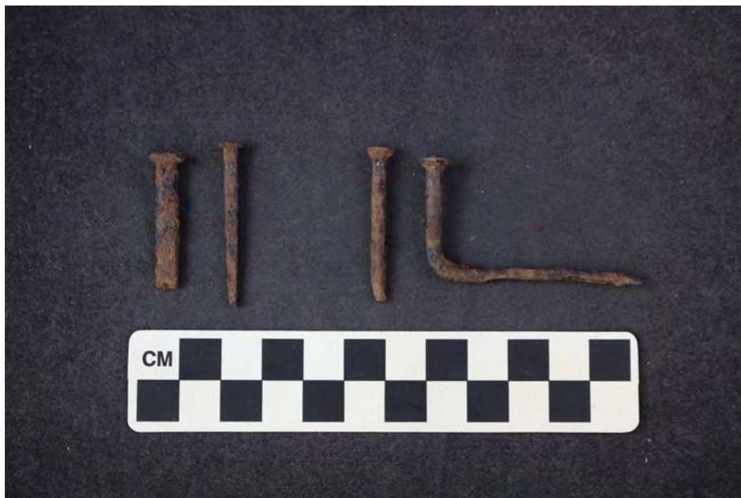
Image 81: Location 7 (AkHa-26); a representative example of nails, (L to R): machine cut (x2), wire drawn (x2).
