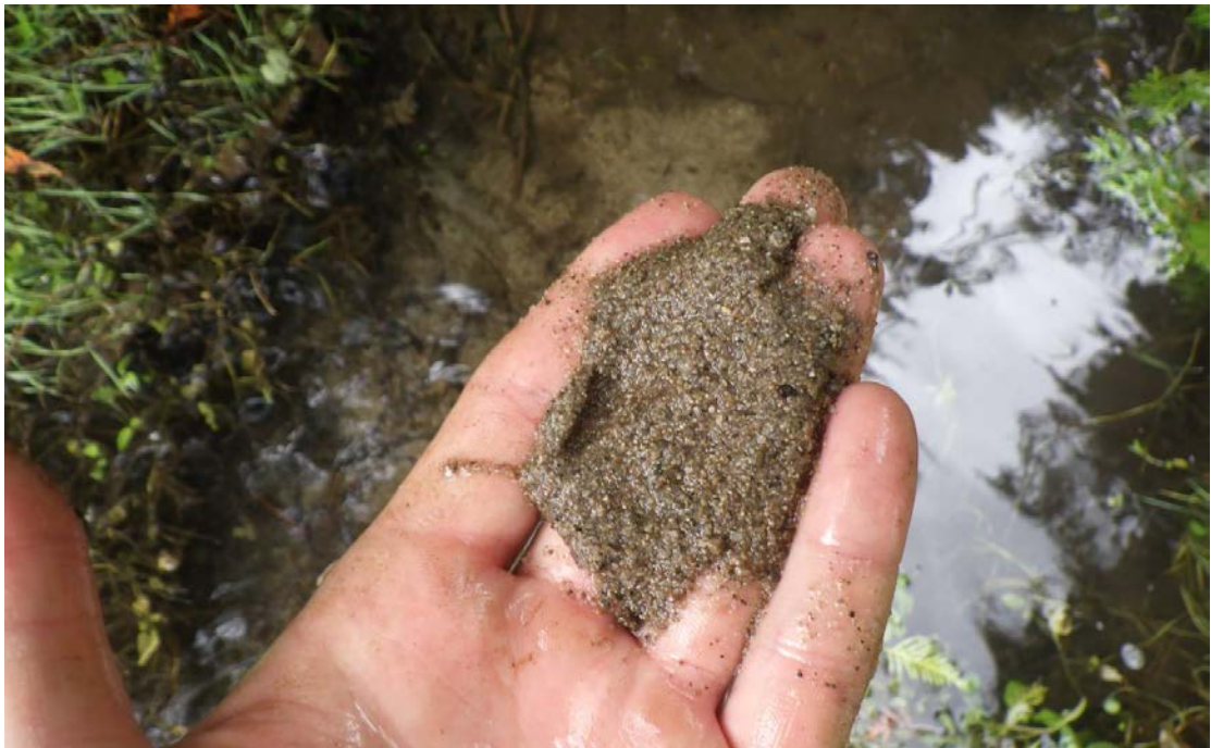
East Ponds Outlet Channel – Bed materials consisted predominantly of medium to very coarse sand.
