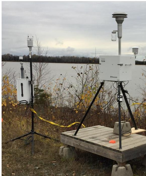
Figure 4: PQ200 and Aeroqual Monitor
