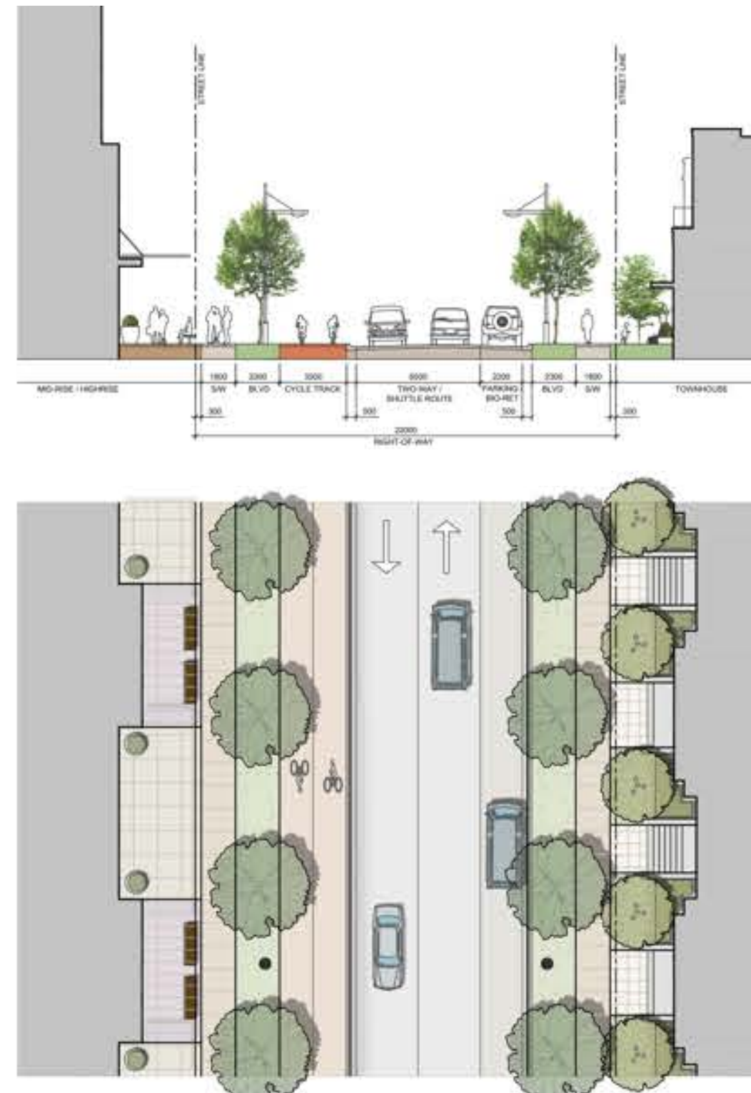
Figure 17: 22.0m ROW - 2 thru lanes; side walk on both sides of the street; on-street parking on one side of the street; separated bicycle track; and street trees in grass boulevard
