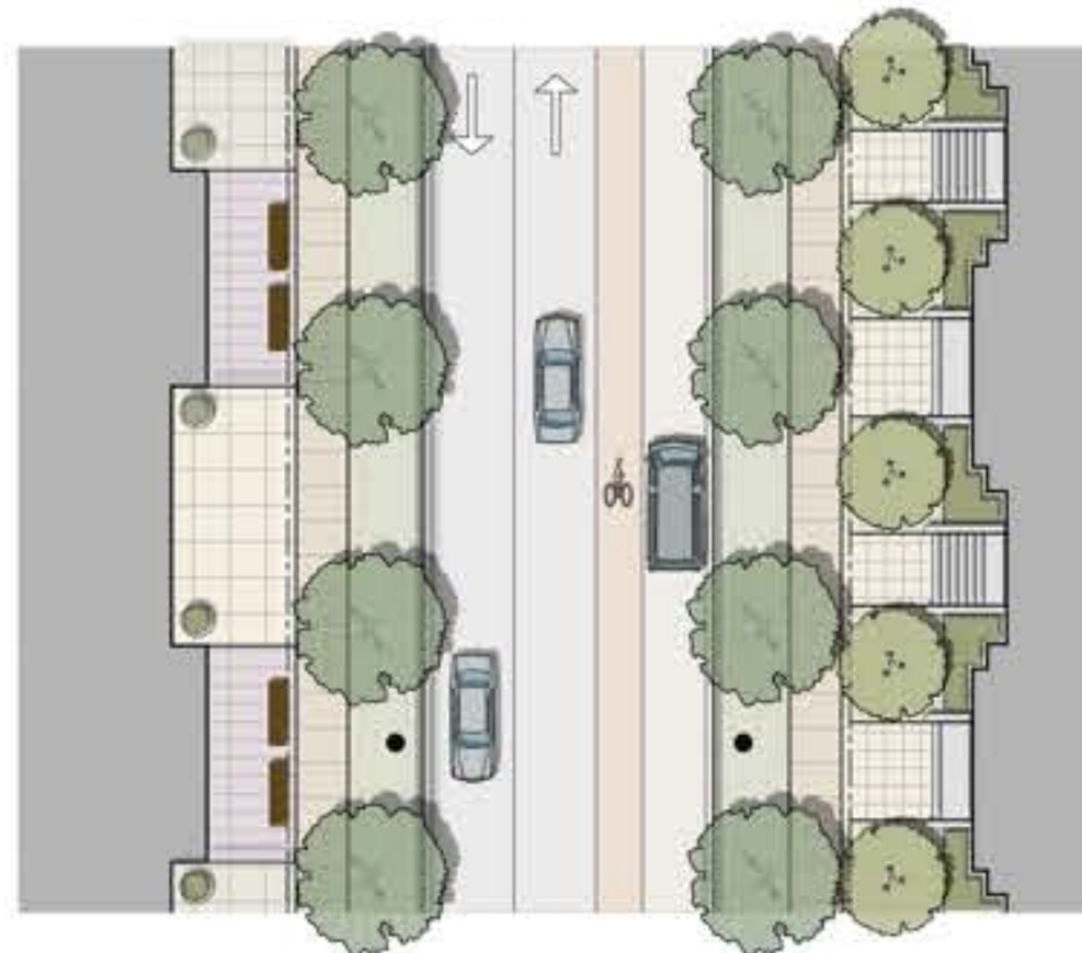
Figure 18: 19.5m ROW - 2 thru lanes; on-street bike lanes; side walk on both sides of the street; on-street parking; and street trees in grass boulevard
