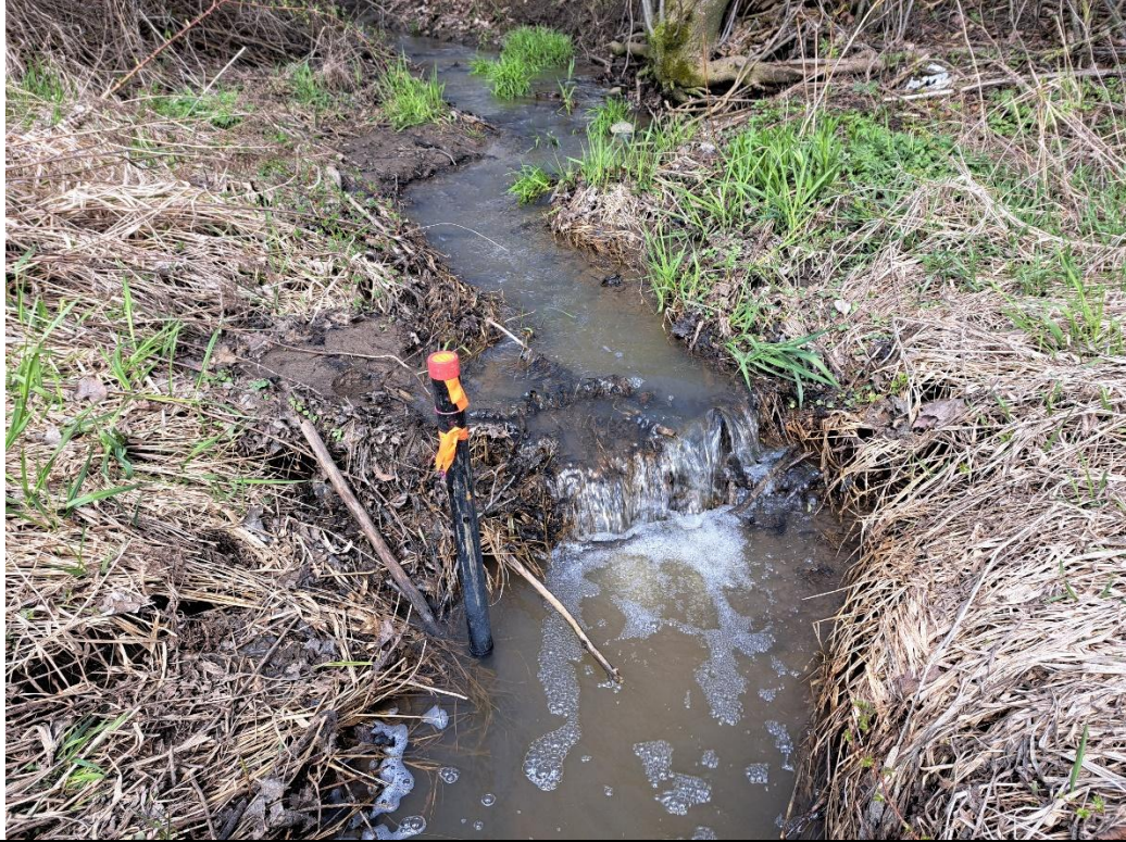
A knickpoint measuring 0.26 m was observed in the downstream portion of the reach. A small pool had formed downstream of the knickpoint.
