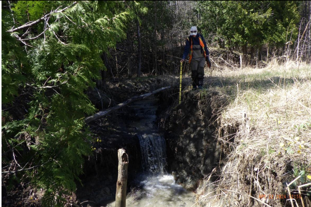
A knickpoint and scour pool were present in the downstream portion of the reach, where increased erosion was also noted.
