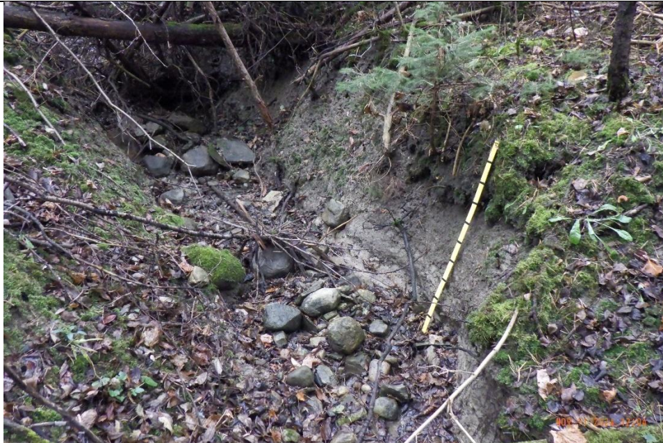
The channel bed substrate ranged from clay/silt to boulders. Channel banks were comprised of clay/silt to gravel.
