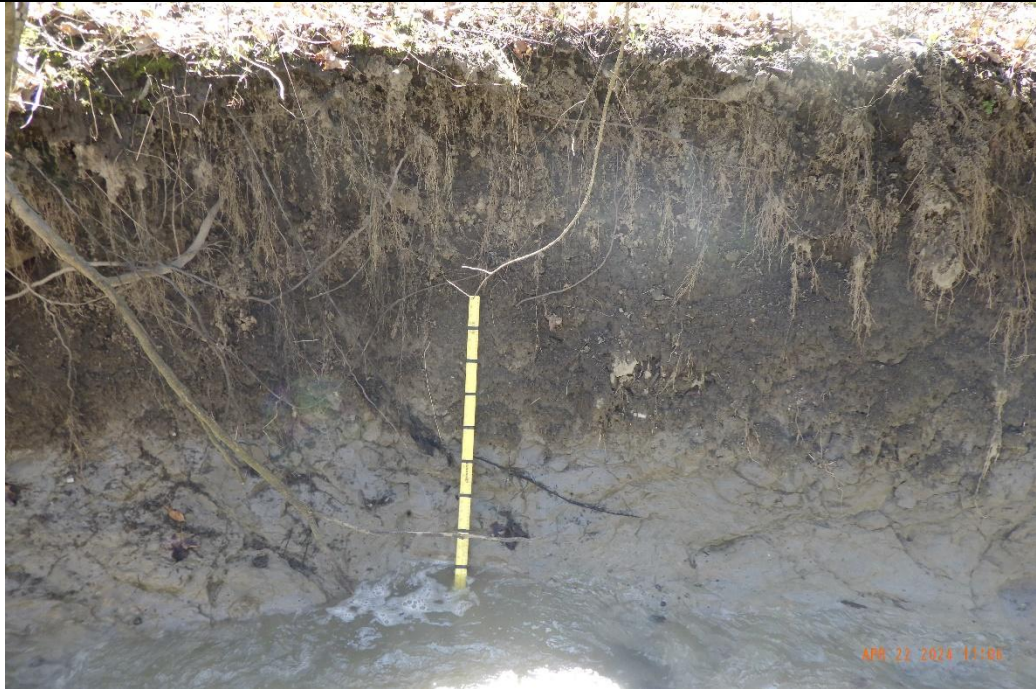
The channel had deeply incised into the clay/till parent material. Bed substrate consisted of till/clay, silt, gravel and cobbles.
