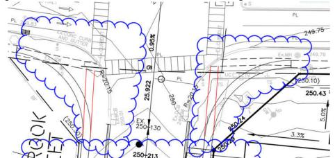
5. The existing utilities are in conflict with the proposed 525mm storm pipe and will need to be relocated. The developer will be responsible for coordinating with utility companies and providing necessary construction designs and details at the detail design stage.
