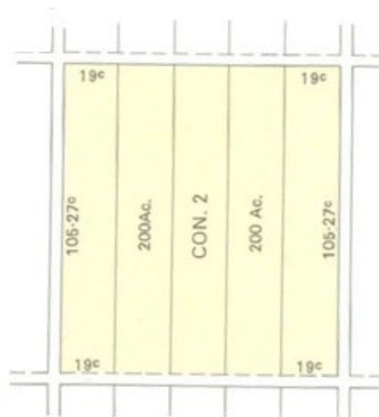
Plate 1: Single Front Survey System (Dean 1969)
