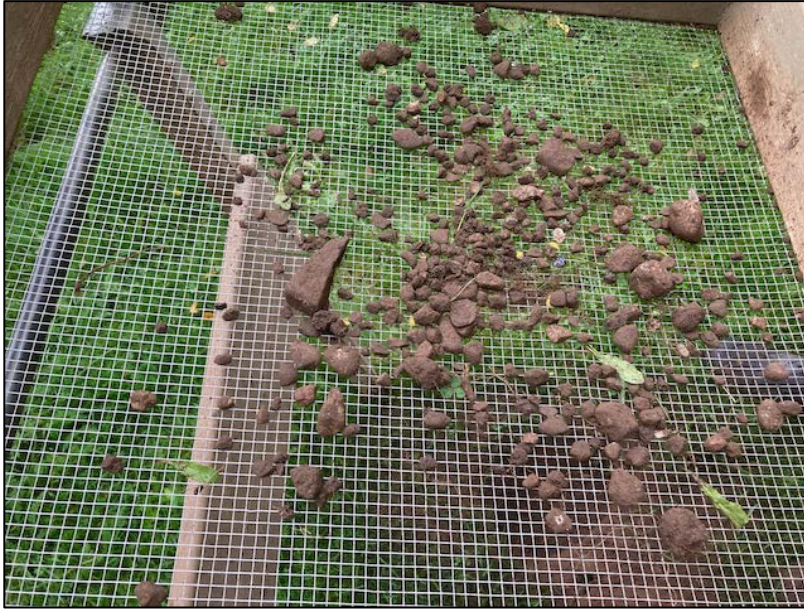
Image 3: Representative image of gravel fills found in disturbed test pits.
