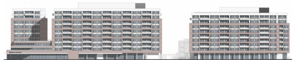
Figure 20 - Site elevation along Columbia Way: the proposed 10-storey building with a 3-storey component at the intersection with Highway 50 and the proposed 9-storey building along Columbia Way
