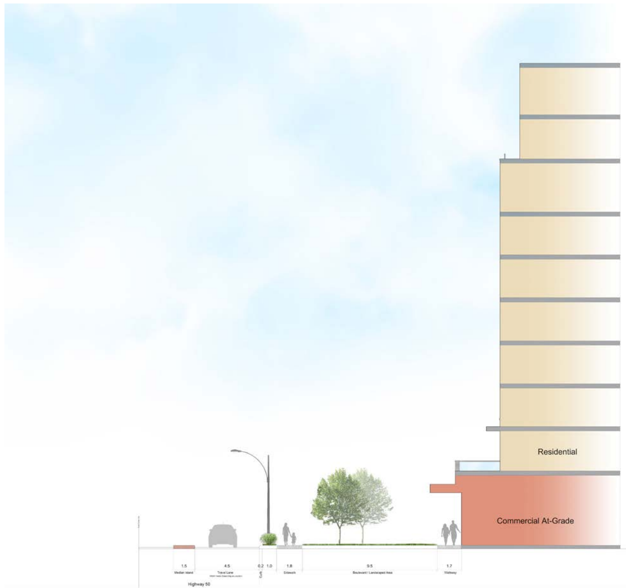
Figure 18 - Conceptual Cross-Section through Highway 50 and Columbia Way. Demonstrates a conceptual condition of the retail interface with the public realm.
