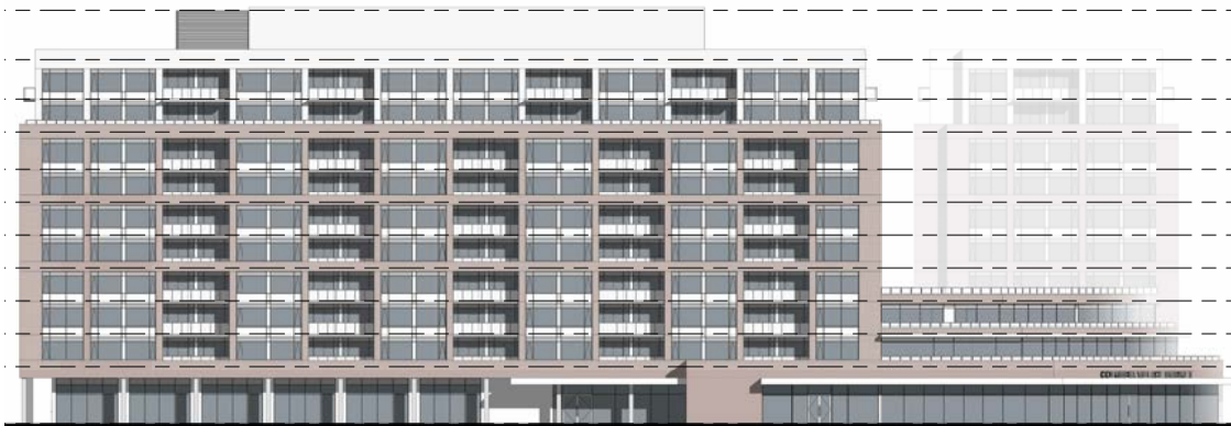
Figure 16 - Phase 2: Proposed Mixed-use Building with retail on the ground floor and apartments above: West Elevation along Highway 50
