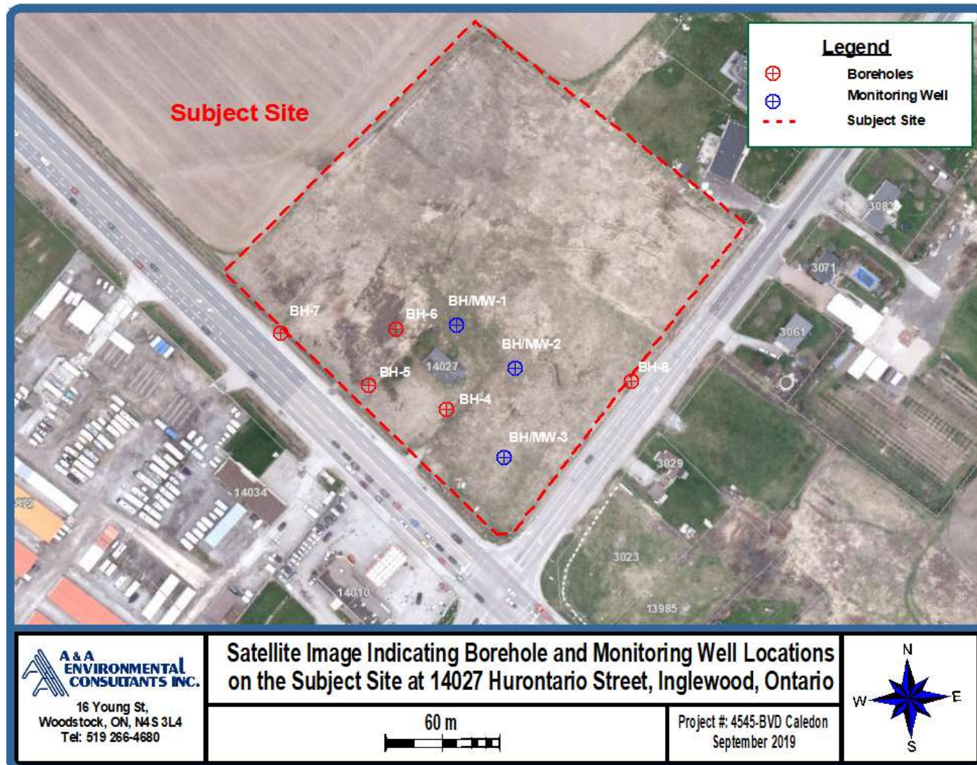
Figure 4 – Geotechnical Boreholes Location, Satellite Image
