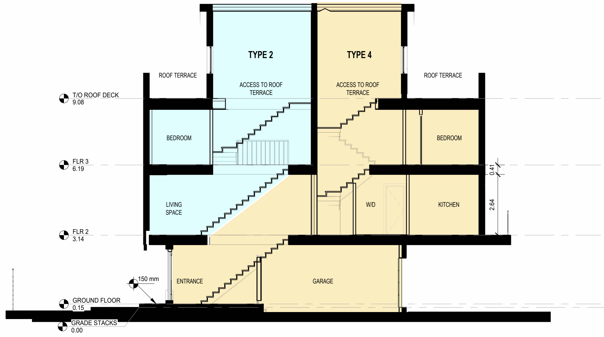
BUILDING 2 CROSS SECTION 1 : 100
