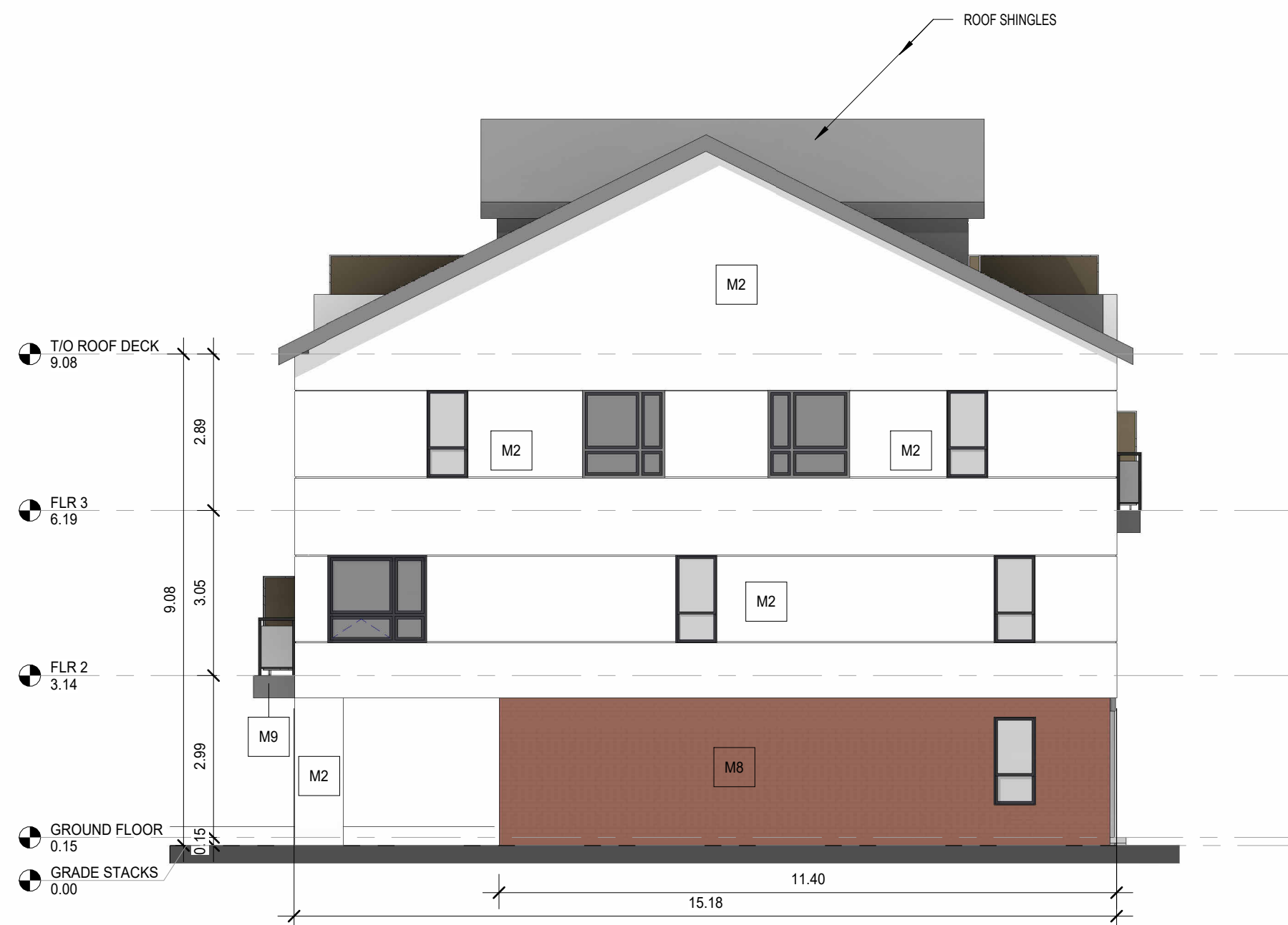
BUILDING 2 - EAST ELEVATION
