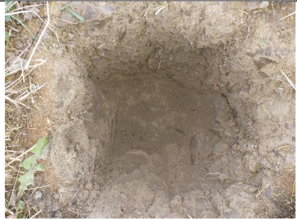
Image 14: Typical test pit.
