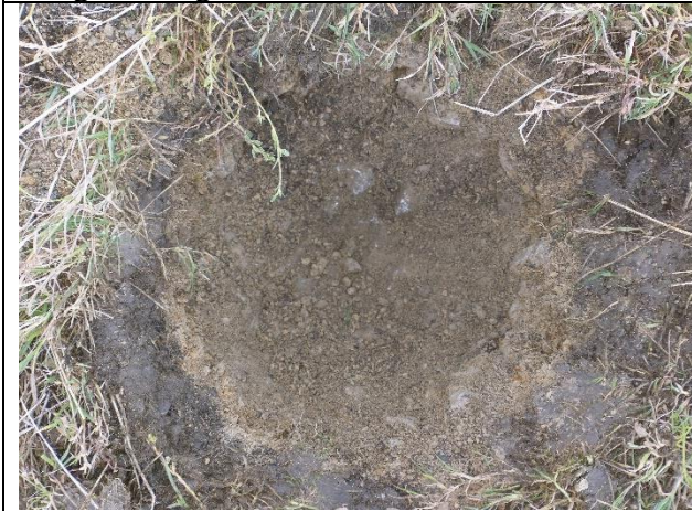
Image 15: Gravel filled test pit.
