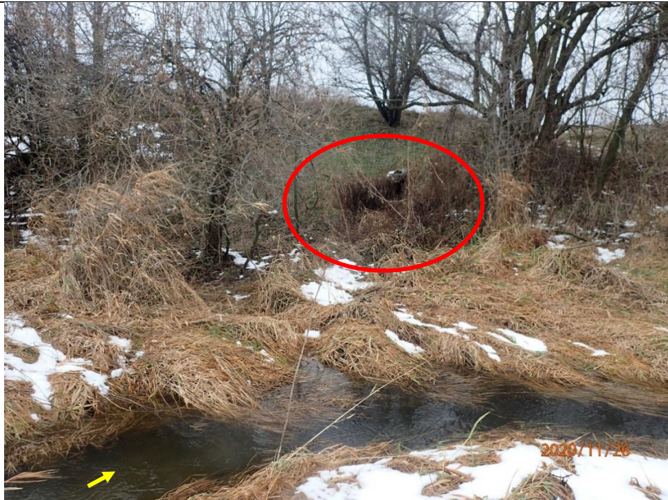
Photograph taken facing valley wall. Approximately 71 – 80% of the bank network was considered stable with infrequent signs of bank slumping or failure (circled).
