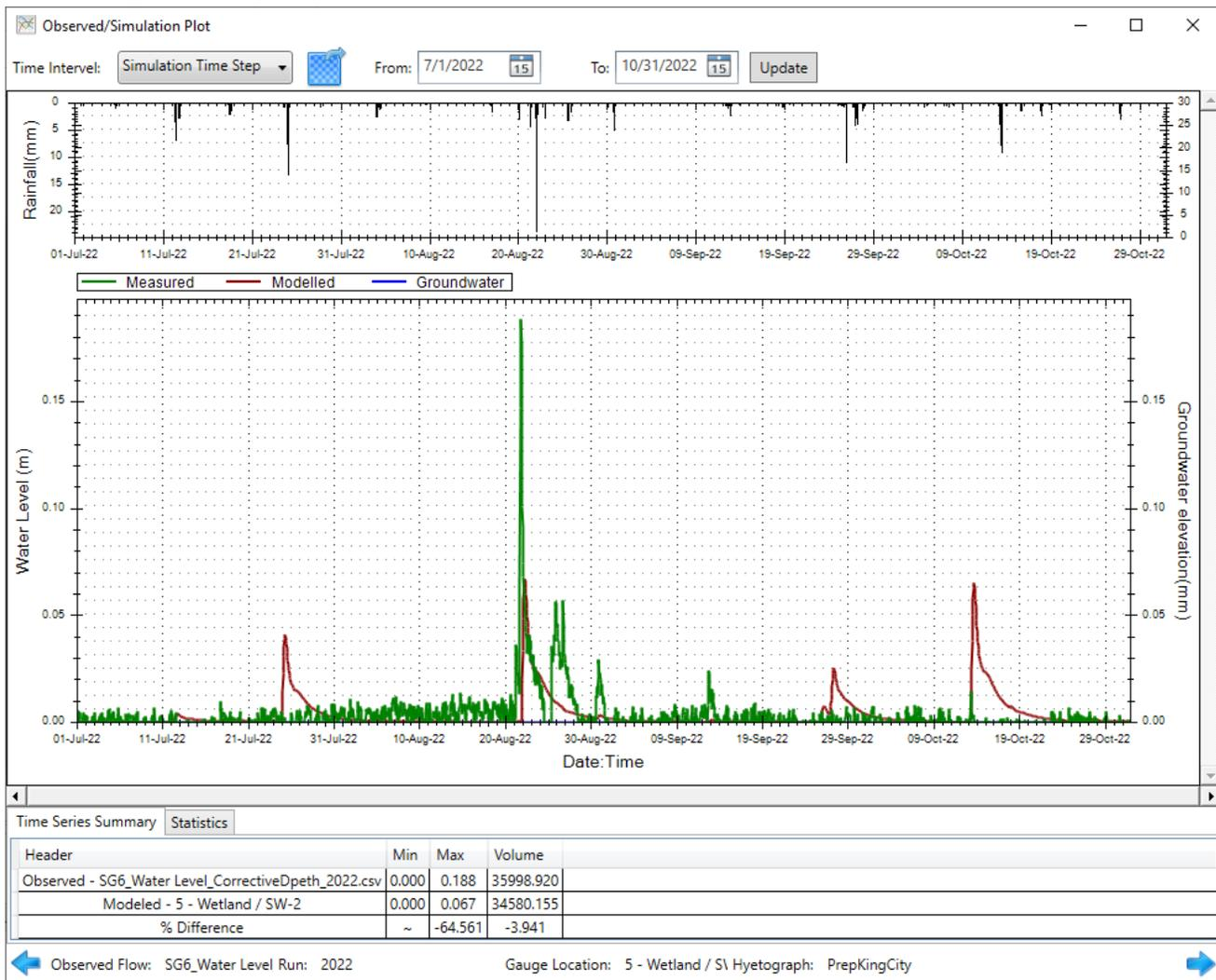
**Illustration 4.2 Comparison of Water Levels for Model Calibration, 2022**
