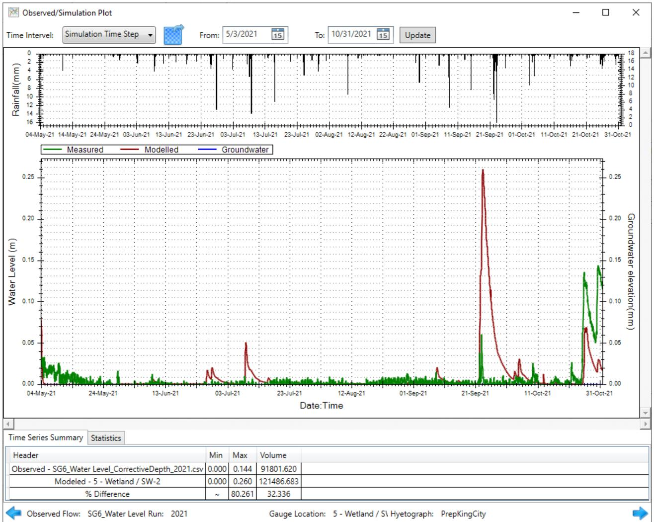
**Illustration 4.1 Comparison of Water Levels for Model Calibration, 2021**
