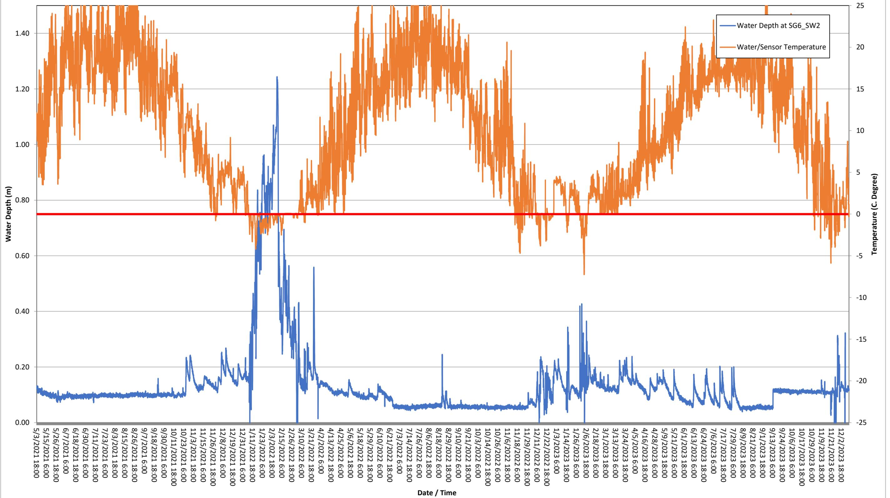
better understand the runoff response in relationship with the rainfall, the corresponding hourly precipitation data was purchased from Environment Canada at its Weather Station of King City (ID 6154150), the nearest station to the study area that has the available hourly weather data for the identified period (e.g., 2021 to 2023). The recorded continuous water levels with precipitation at SW-2 (SG6) are plotted in **Figure 3.2**.
