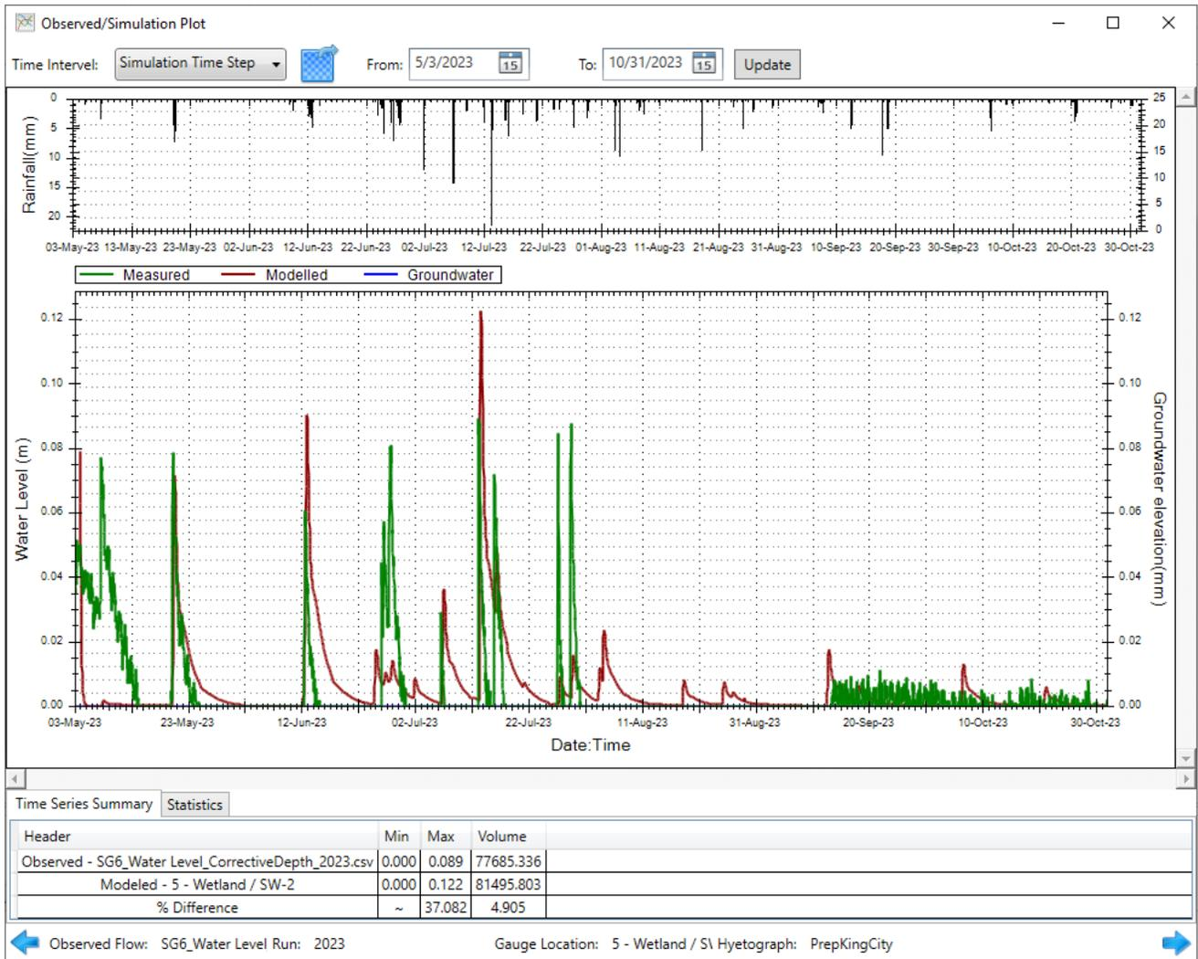
**Illustration 4.3 Comparison of Water Levels for Model Calibration, 2023**
