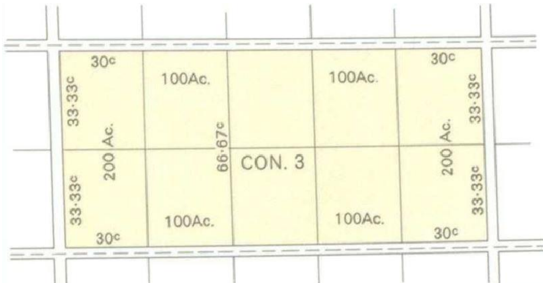
Plate 1: Double-Front Survey System (Dean 1969)
