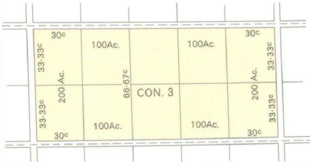
Plate 1: Double Front Survey System (Dean 1969)
