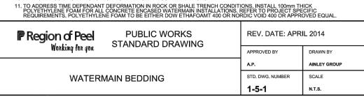
8. MIN. TRENCH WIDTH TO BE O.D. PLUS 600mm MAX. TRENCH WIDTH TO BE O.D. PLUS 750mm, UNLESS PROJECT SPECIFIC BEDDING STATES OTHERWISE.
