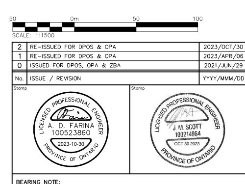
BEARING NOTE: BEARINGS ARE UTM GRID, DERIVED FROM GPS OBSERVATION USING THE "TOPNET" GPS NETWORK OBSERVATIONS, UTM ZONE 17, NAD83 (CSRS) (2010.0) & (1997.0). SURVEY COMPLETED BY YOUNG & YOUNG SURVEYING INC. & J.D.BARNES LIMITED DATED 2021/OCT/07, 2021/OCT/14 & 2018/NOV/28, PROJECT Nos. 21-B7601-4, 21-B7601-5 & 18-30-308-00-A.
