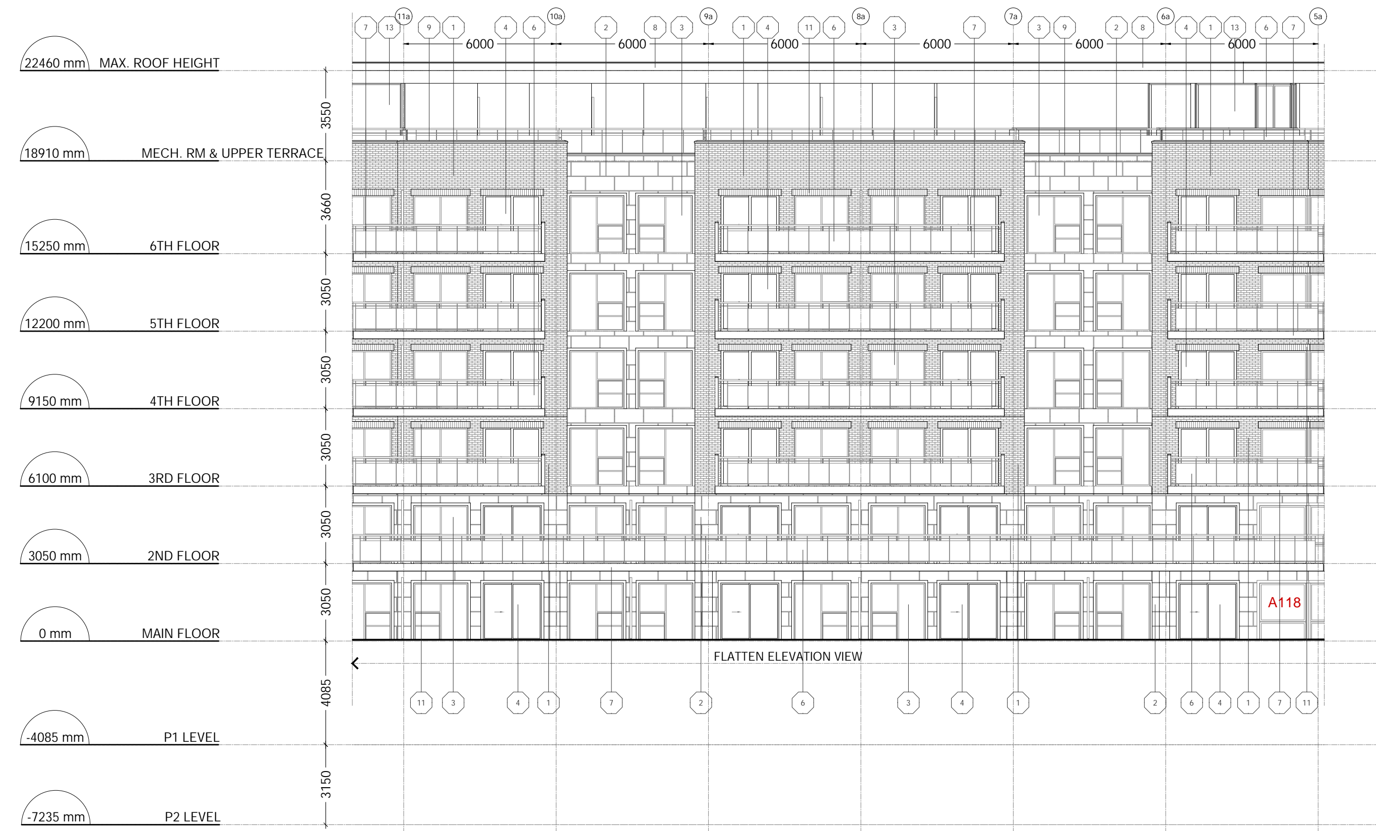
1 WEST ELEVATION - TOWER A A3.0 SCALE: 1:150
