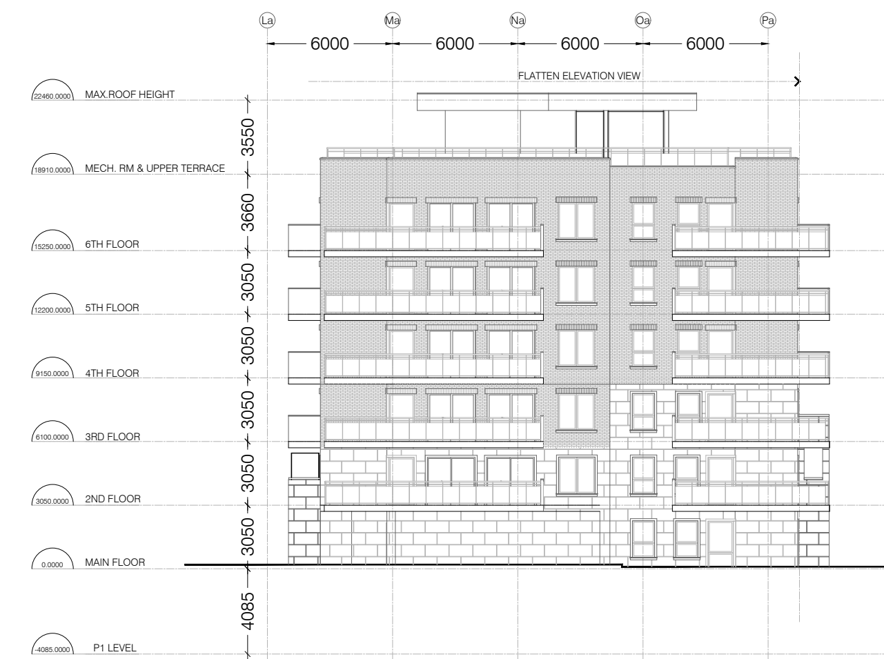
6 NORTH ELEVATION - TOWER A A3.0 SCALE: 1:250
