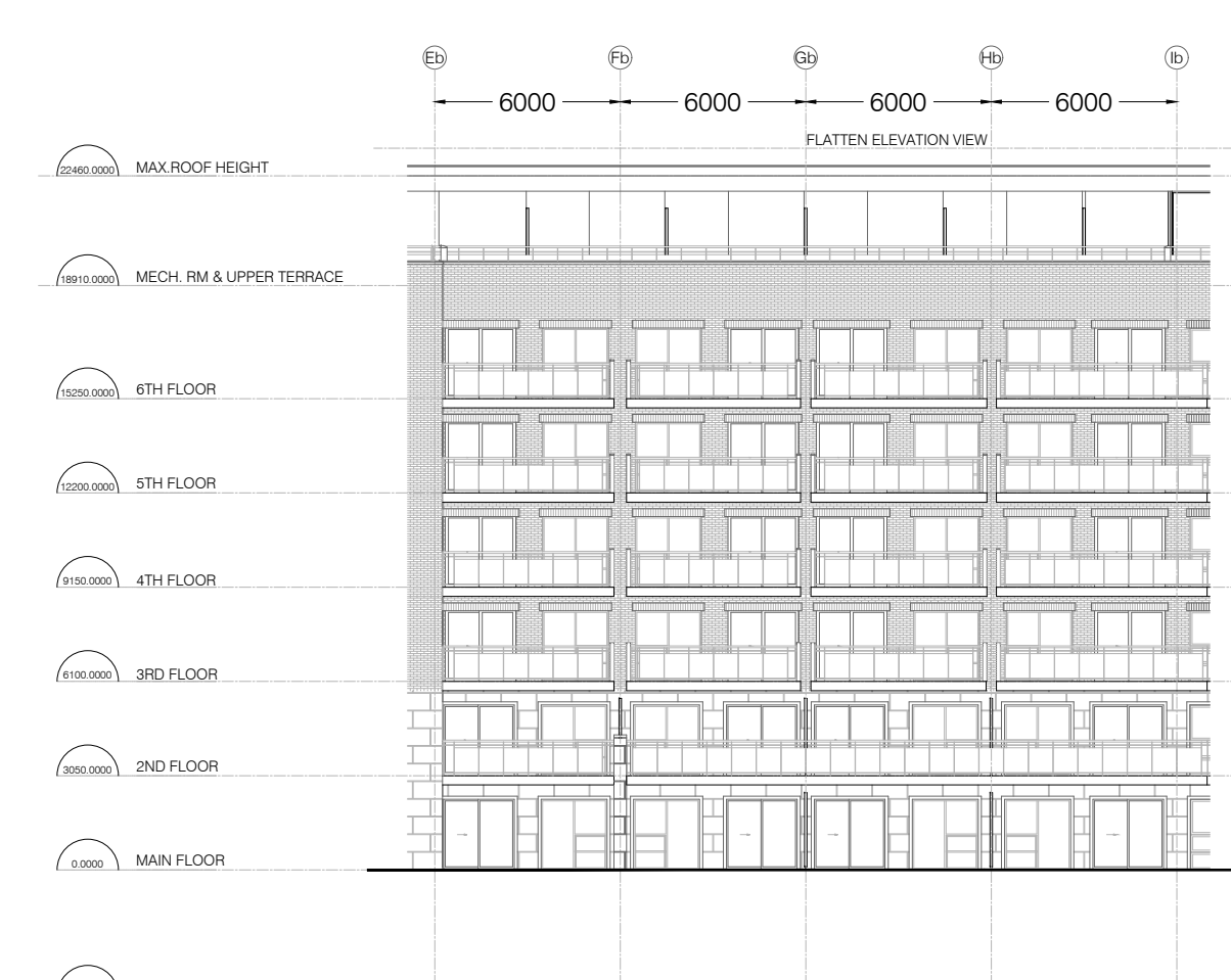
5 NORTH ELEVATION - TOWER B A3.1 SCALE: 1:250
