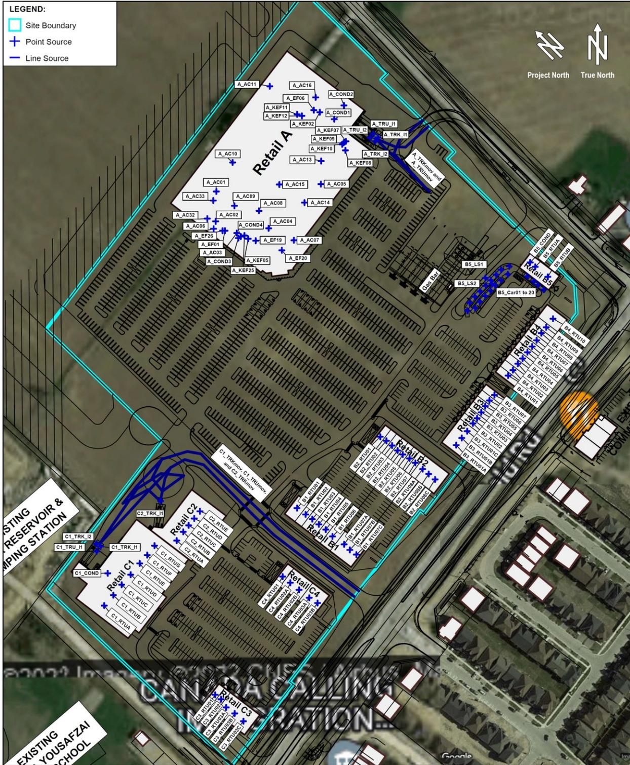
FIGURE 2A: SITE PLAN AND NOISE SOURCE IDS & LOCATIONS – NON-IMPULSE SOURCES
