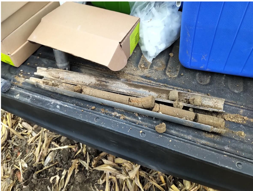
Photograph No. 10 – View of the clayey silt till observed at borehole BH135-20.
