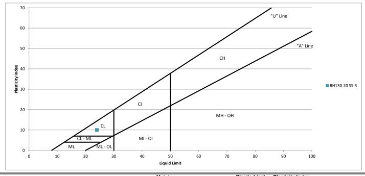
Plastic Limit Plasticity Index Moisture Liquid Limit (W<sub>L</sub>) **Borehole** Sample # Sample Depth (I<sub>P</sub>) Content (%)  $(W_P)$ BH130-20 24 SS-3 1.5-2.1 mbgs 11
