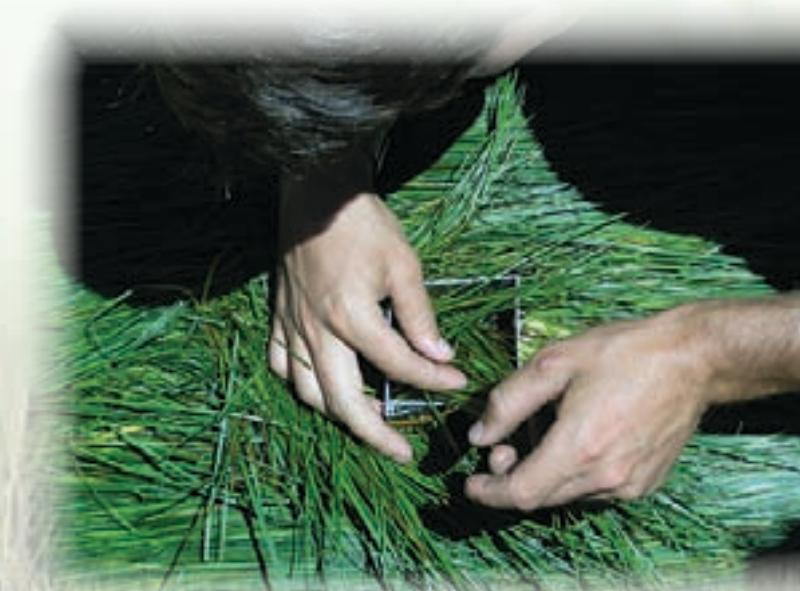
At the completion of the test, an extracted soil sample showed vegetative root penetration to a depth of 1.5 inches (38 mm), with larger roots interacting with the cell wall perforations. As future growth occurs, root interaction will increase.
