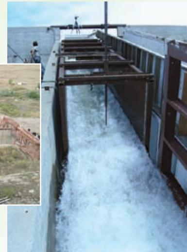
subjected to flow discharges ranging from 10 ft/sec (3.0 m/sec) to 27 ft/sec (8.2 m/sec). Two sets of water surface elevation data were taken; one at the beginning and one at the end of each hour-
