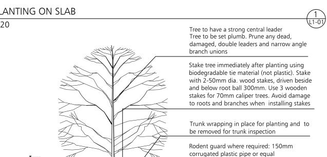
Cut and remove wire, burlap and twine from trunk and top 1/2 of rootball. Remove all ties from collar of plant Set top of root ball 50mm minimum above finished grade. For poorly drained soil, see note below. Provide topsoil saucer 100mm above finished grade. Pit and suacer to be soaked with
