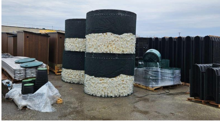
Waterloo Biofilter System - Filter Medium (Guelph, Ontario manufacturing facility)
