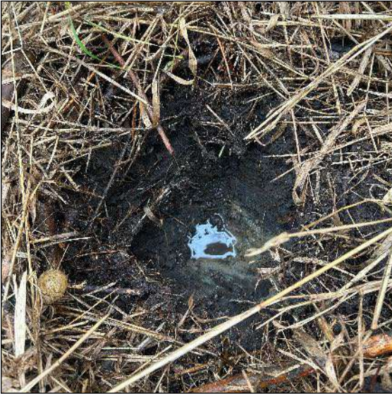
Image 21: Test Pit to confirm limit of Low Lying & Wet lands, note gley soil.
