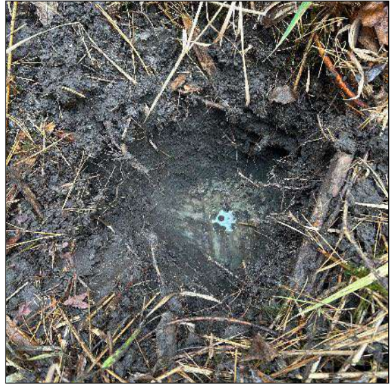
Image 22: Test Pit to confirm limit of Low Lying & Wet lands, note gley soil.
