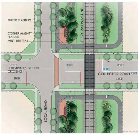
PRELIMINARY CONCEPTUAL SKETCH OF THE PROPOSED STREET CROSSING OF THE RAILWAY LINE WITH ASSOCIATED PLANTED BUFFERS AND CORNER FEATURES.
